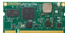
VAR-SOM-AM62 TI AM625X 4X 1.4GHZ CORTEX-A53
